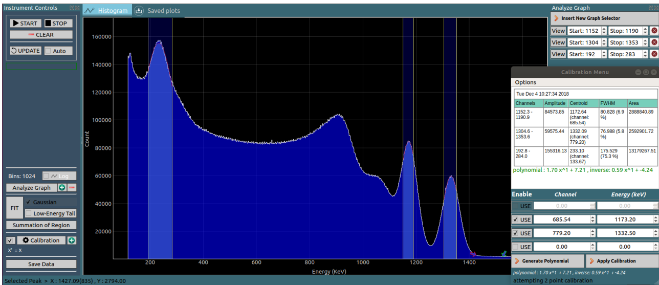
Figure 6: Gamma Spectrum from Cobalt-60
