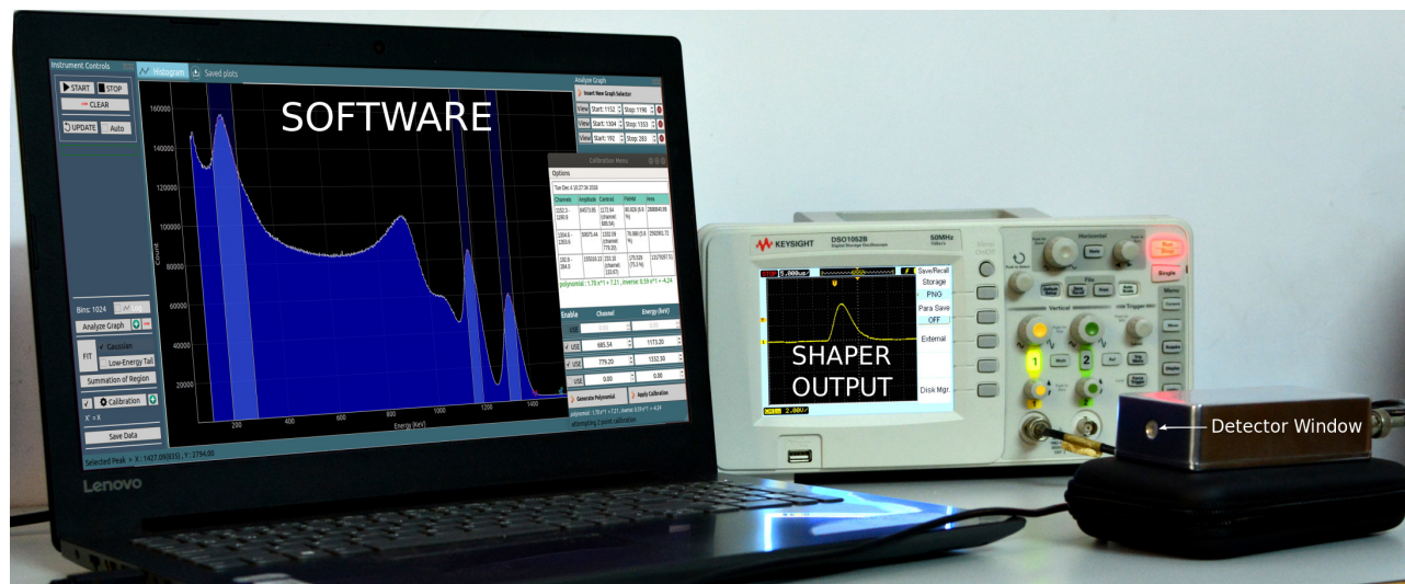
Figure 2: Entire experiment setup of the Gamma Spectrometer 'GammaSpec-1K'. Also shown is a laptop connected via the USB port with an example spectrum. Signal outputs from the shaping amplifier are connected to a 50MHz oscilloscope where the nature of this signal is shown
