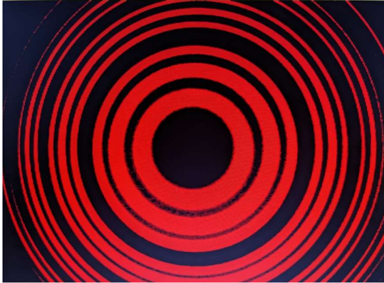
Fig.6 Pattern recorded with lab setup for Normal Zeeman effect after alignment
